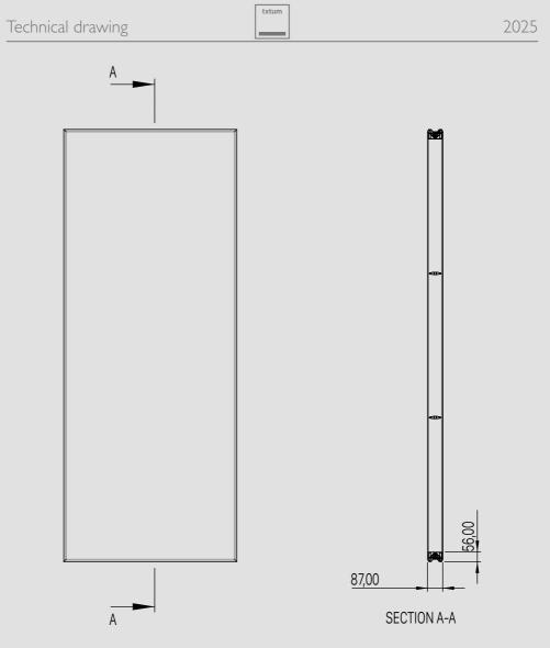
**STRUCTURE:** supporting structure in extruded aluminium on 4 sides.
