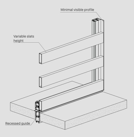
**PERPENDICULAR DIMMING:** from 100% to 0% (depending on the slats and the pitch of the slats).
