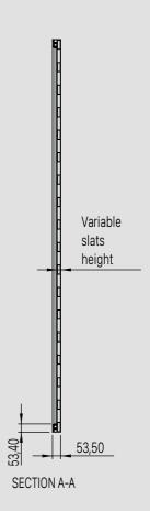
**STRUCTURE:** supporting structure in extruded aluminium on 4 sides.
