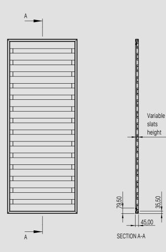
**STRUCTURE:** supporting structure in extruded aluminium on 4 sides.
