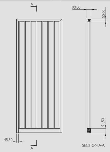
**STRUCTURE:** supporting structure in extruded aluminium on 4 sides.
