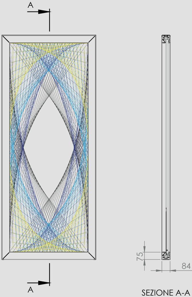
**STRUCTURE:** supporting structure in extruded aluminium on 4 sides.
